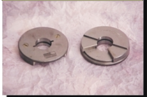
GO Gauges for B22 Bayonet Cap
